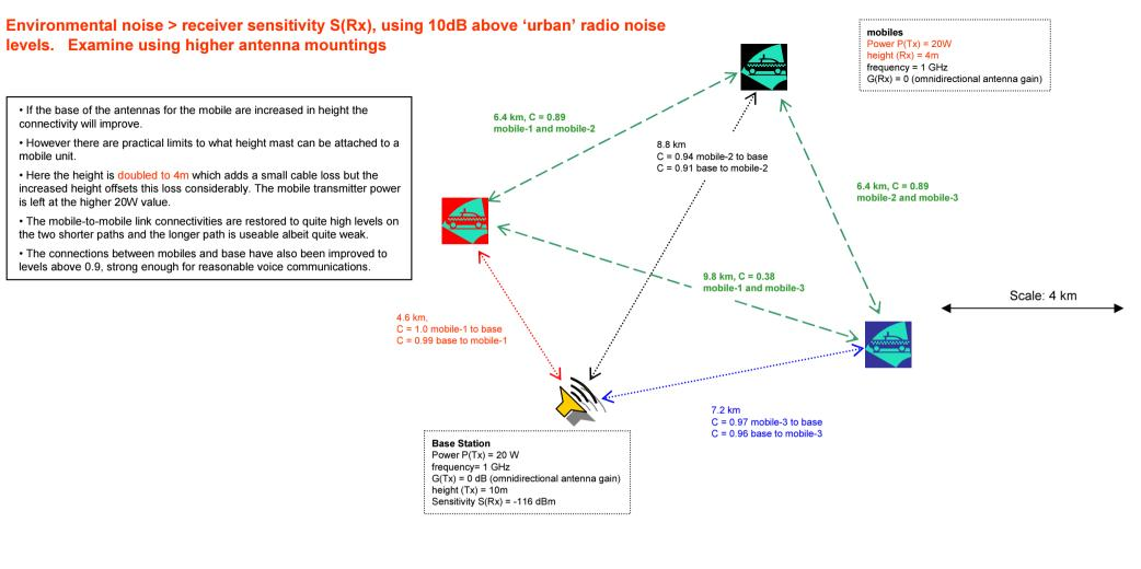
Network Connectivity using higher antenna mountings
